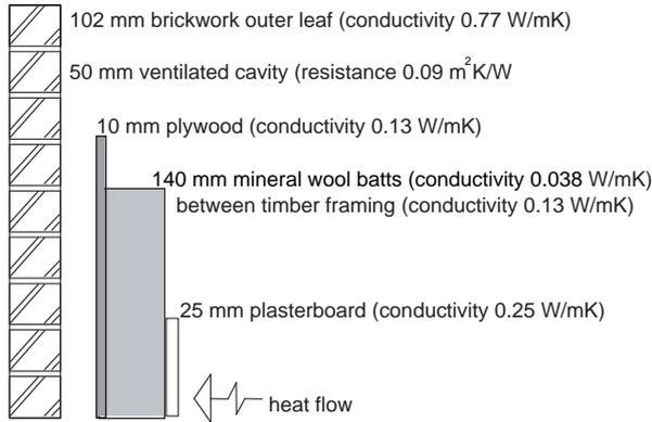
(Total thickness 327mm,  $U = 0.30\text{W/m}^2\text{K}$ )
