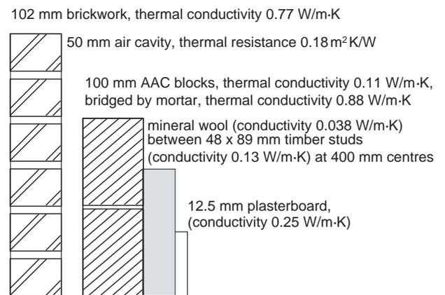
(Total thickness 353.5mm,  $U = 0.32 \text{ W/m}^2\text{K}$ )
