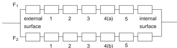
**Resistance through the section containing insulation**
