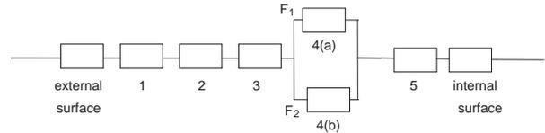
The lower limit of resistance is then obtained by adding up the resistances of all the layers:
