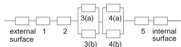
The resistances of the layers are added together to give the lower limit of resistance. The resistance of the bridged layer consisting of AAC blocks and mortar is calculated using:
