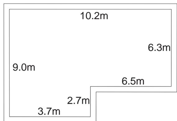
The perimeter to area ratio is equal to  $(38.4/74.25 = 0.517) \text{ m/m}^2$ . Table C1 provides values for perimeter/area ratios of 0.50 and 0.55 but not for any values between 0.50 and 0.55. In this case, the U-value corresponding to a perimeter to area ratio of 0.50 should be used since 0.517 is closer to 0.50 than to 0.55.
