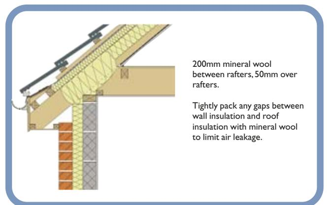
Figure 5: Pitched roof with insulation between rafters
