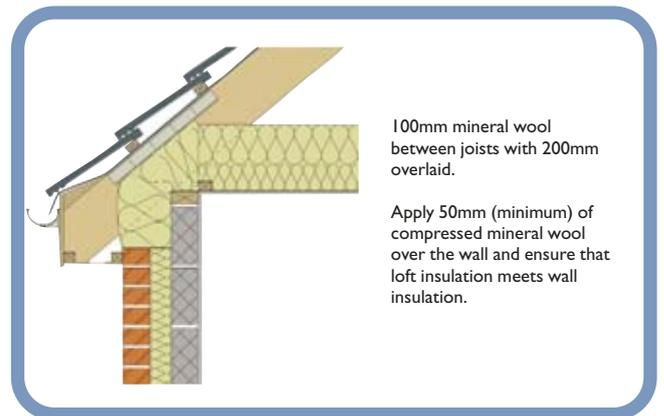
Figure 4: Pitched roof with insulation between joists
