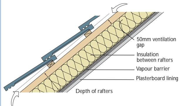
**Figure 11: An unventilated insulated pitched roof with vapour balanced or 'breathing' construction, and incorporating insulation between rafters**
