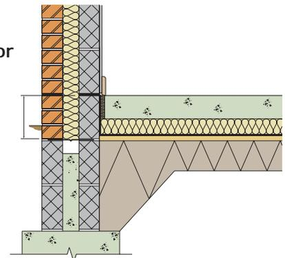
**Figure 4: Insulating a concrete floor above the slab**
