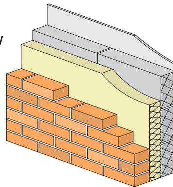
Timber-framed construction usually consists of a structural timber frame with insulation placed between the framing members, lined internally with plasterboard and externally with a sheathing board and a waterproof breather membrane. The timber frame is often clad externally with a skin of brickwork, separated from the frame by a cavity (see Figure 8). Timber frames are usually either 90mm or 140mm thick. In order to meet the Best Practice standard it is necessary to:
