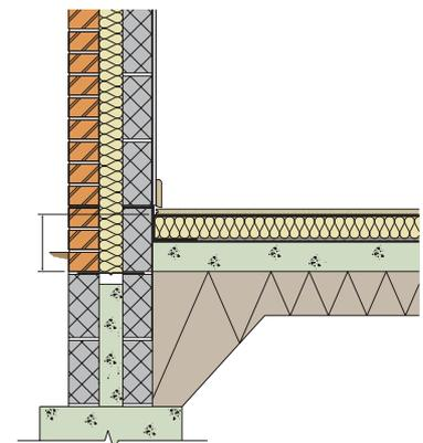
Suspended pre-cast concrete 'beam and block' floors are usually insulated above the floor, as shown in Figure 5. Again rigid insulation should be used. The thickness of the insulation should not exceed about 100mm, so a high performance insulating material (i.e. one with low thermal conductivity) may be required to meet the Best Practice standard.
