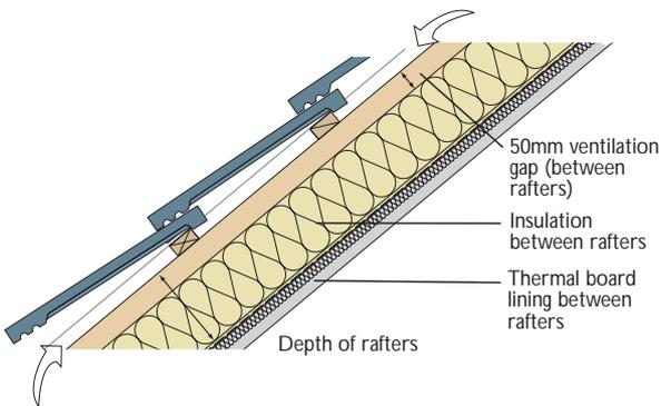
**Figure 8: An unventilated insulated pitched roof with vapour balanced or 'breathing' construction, and incorporating insulation**
