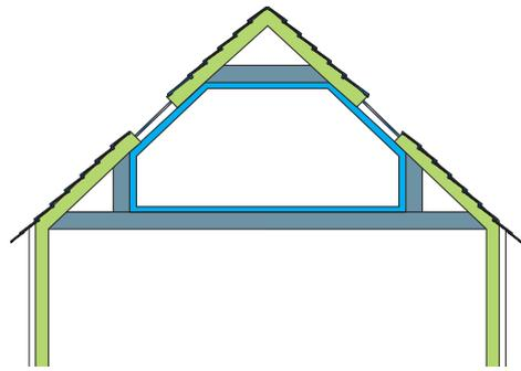
Figure 2: Insulating a 'dormer' type conversion (option 2)
