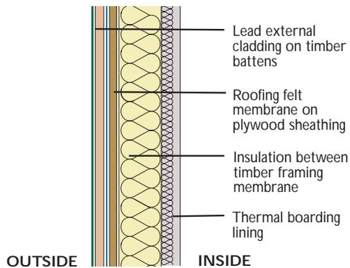
**Figure 11: Insulating exposed gable walls internally using a proprietary insulation board**
