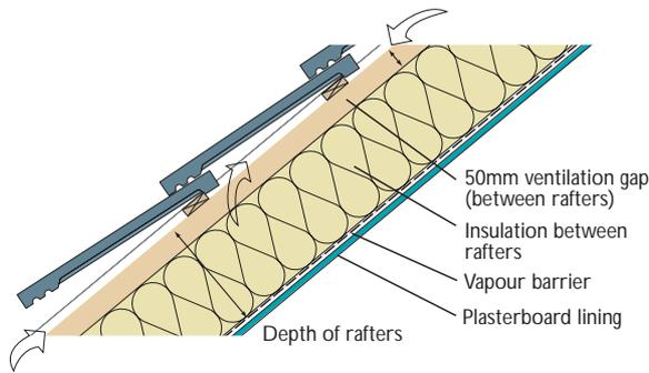
**Figure 7: A ventilated pitched roof, with insulation between rafters supplemented by a ceiling lining of thermal board**
