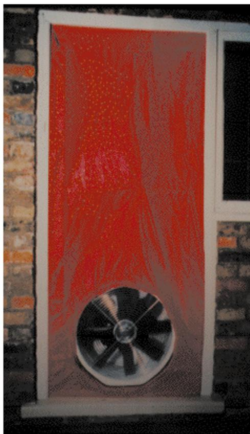
*Figure 7 The fan pressurisation technique employs a fan fitted in a dummy door panel*
