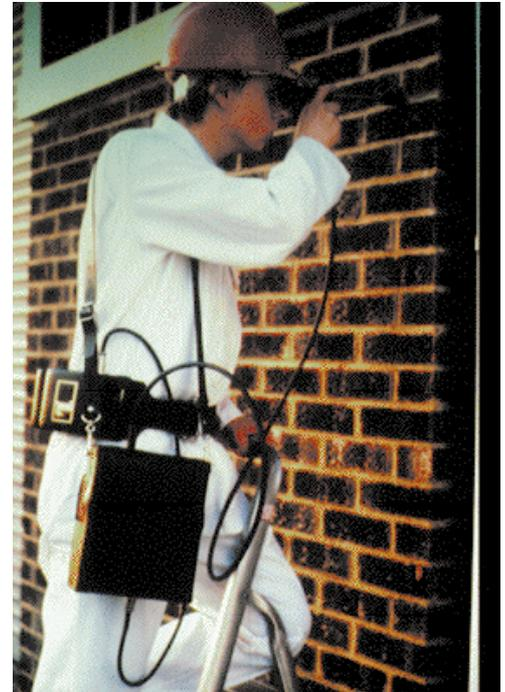
*Figure 10 Borescope examination of wall cavity*
