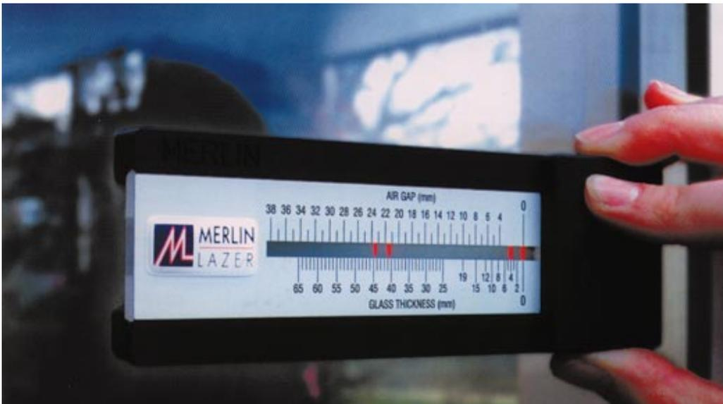
*Figure 8 Laser gauges provide a simple way of identifying the type of glazing installed within a window*
