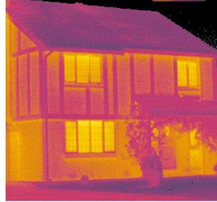
*Figure 5 A thermogram of a typical house, highlighting areas of relatively low insulation, such as windows, and the high levels of insulation in the roof space and wall cavities*
