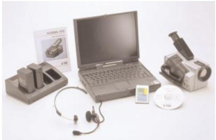
*Figure 6 Thermographic survey equipment*
