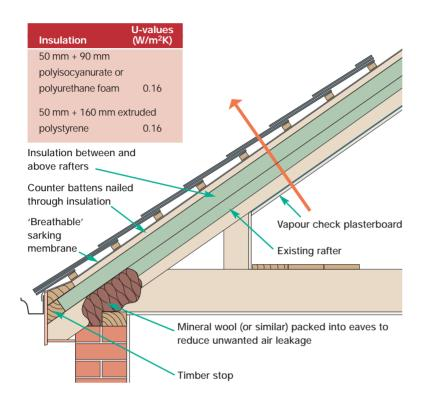
This method of insulating the roof is for use when the existing roof tiling is being renewed.
