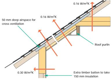
U-values assume timber rafters are at 400 mm centres Note: an uninsulated roof has a LI-value of 1.9 W/m<sup>2</sup>K
