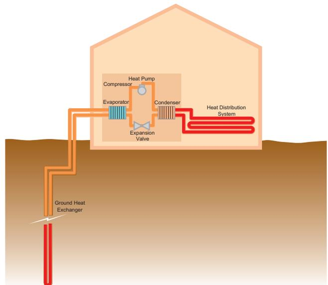
Figure 4: A typical ground source heat pump system
