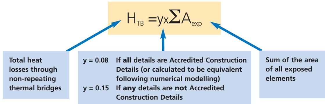
This second approach means that the heat loss due to thermal bridging can be estimated by simply using the y-value and the total area of exposed elements. Previously only two default y-values were available:
