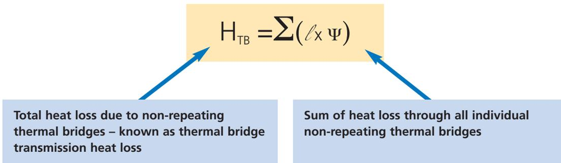
If the design uses ACDs<sup>4</sup>, or ACDs (Scotland)<sup>5</sup>, a set of default  $\Psi$ -values (table 1) can be used. Alternatively, if ACDs are not being used, the calculation of their  $\Psi$ -values and temperature factors should be determined from numerical modelling (in accordance with BR 497)<sup>6</sup> or from measurement.
