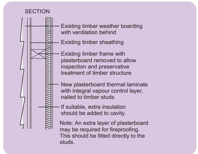
Figure 2: Timber framed external wall with plasterboard laminate
