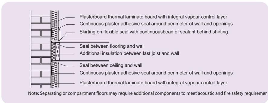
Figure 6: Timber stud frame in existing flats
