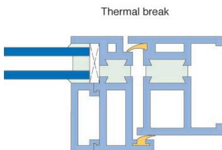
Figure 4: Section of metal window showing thermal breaks
