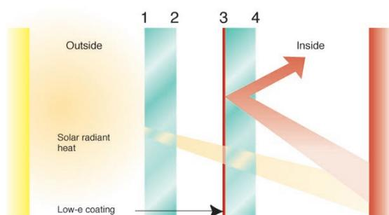
Figure 1: The low-e coating on Surface 3 reflects longer wavelength radiation back into the room, reducing heat loss
