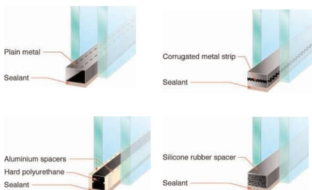
Figure 2: Conventional plain metal and 'warm edge' insulating spacer bars
