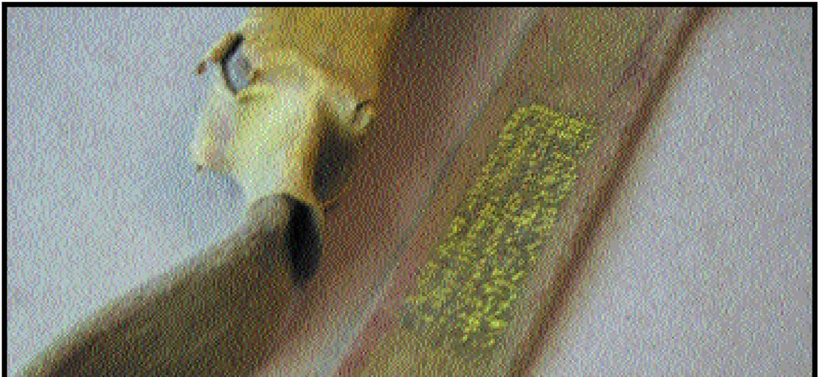
**Missing label: damage to protective sleeve over energy absorber**
