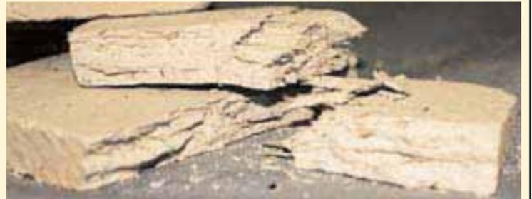
**Asbestos insulating board** is very dangerous material. Asbestos fibres can easily be released if it is disturbed - only specialist-licensed contractors can remove it.
