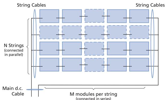
For a system of N parallel connected strings, with each formed of M series connected modules, string cables are to be rated as follows:
