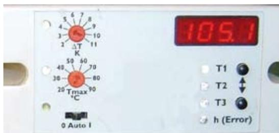
Figure 12 Differential thermostat
