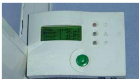
Figure 13 Differential thermostat
