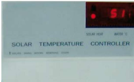
**Figure 14** Differential thermostat
