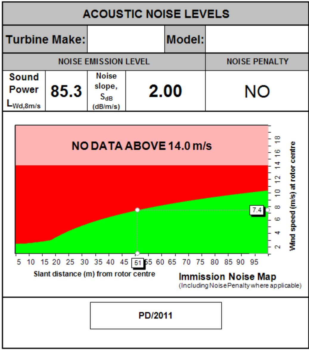
The noise map can be read by drawing a horizontal line from the recorded wind speed at hub (right hand side of the map) to where the red and green lines meet. Drawing a vertical line from this point to the bottom of the map will give the maximum slant distance in metres from rotor centre (hub) at which a wind turbine could be installed to stay within the noise range. For clarity, MCS Contractors must draw a single line that is no greater than the thickness of a standard biro.
