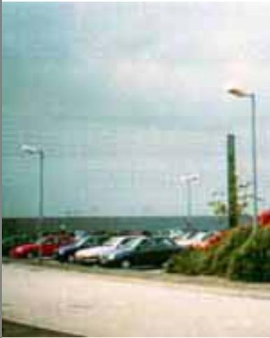
*Magna Park: the new lighting scheme at the Merck site has high pressure sodium lamps with full horizontal cut-off.*
