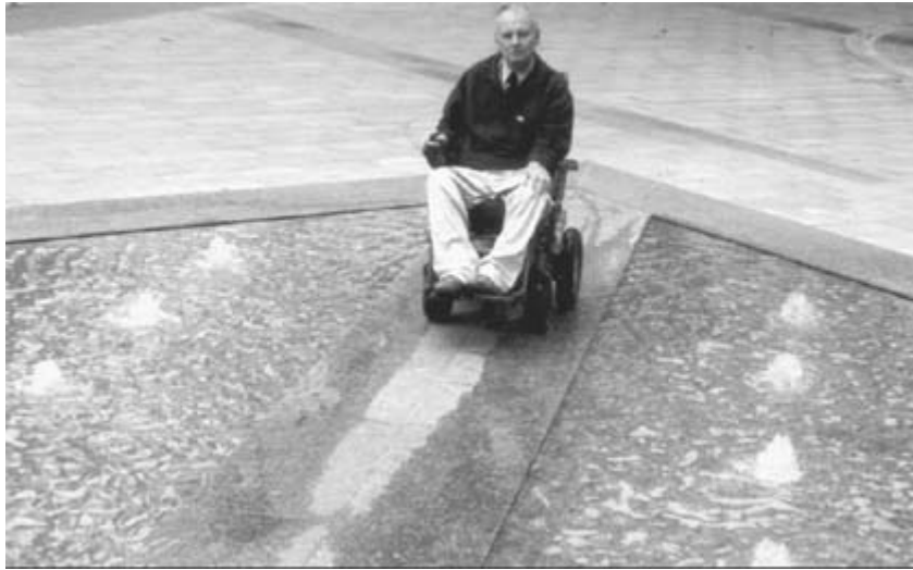
A hard landscape design with a walk-through option for use by all. The texture's tactile surround defines the wet boundary of the feature.
